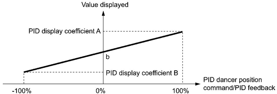
If the sensor output is unipolar, PID dancer control operates within the range from 0 to  $+100\%$ , so virtually specify the value at  $-100\%$  as coefficient B.
