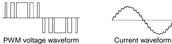
Figure 1.2 Output Voltage and Current Waveform of the Inverter
