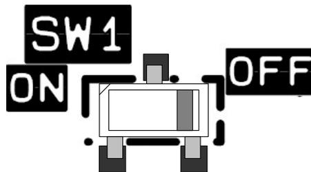
Figure 4.15 Z-phase Wire Break Detector ON/OFF Switch (SW1)
