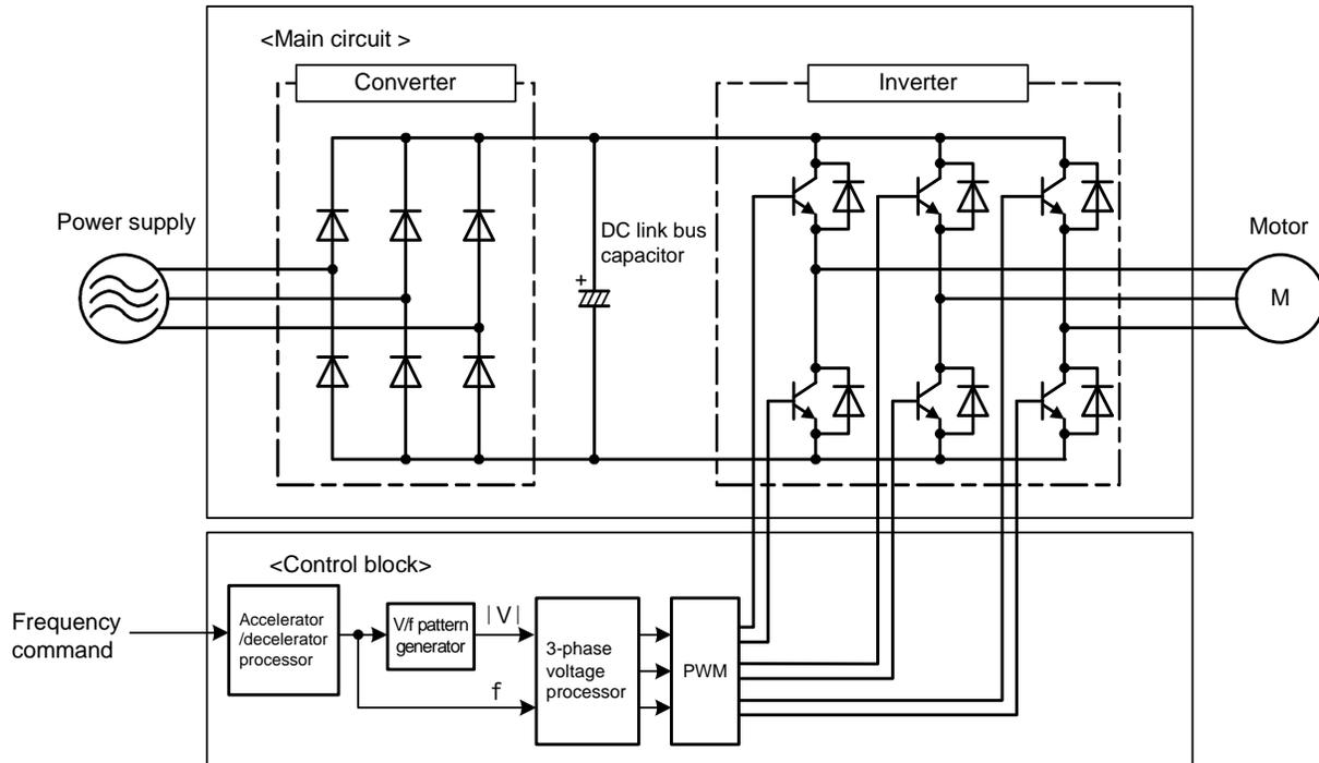
Figure 1.1 Schematic Overview of Theory of Inverter
