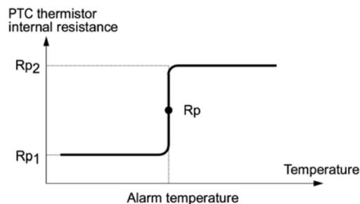
Suppose that the internal resistance of the PTC thermistor at the alarm temperature is  $R_p$ , the detection level (voltage)  $V_{C1}$  is calculated by the expression below. Set the result  $V_{C1}$  to function code H27.
