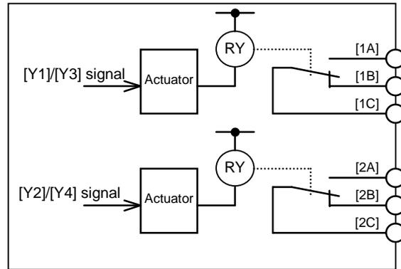
Figure 4.16 Internal Circuits
