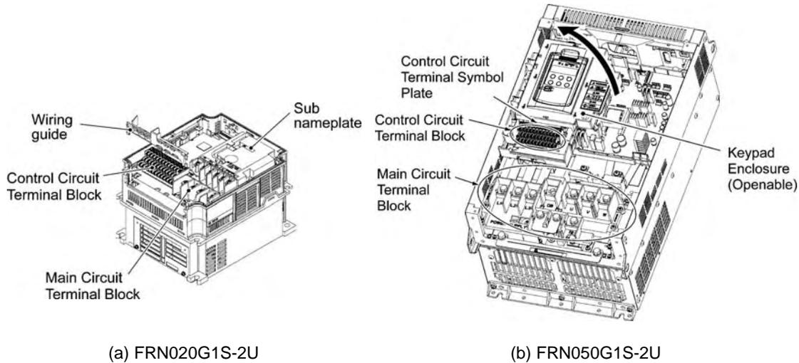
Figure 1.5 Terminal Blocks and Keypad Enclosure Location
