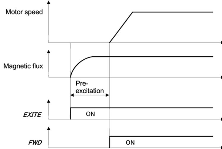
**Note** Under V/f control (including auto torque boost and torque vector), pre-excitation is disabled, so use DC braking or hold the starting frequency instead.
