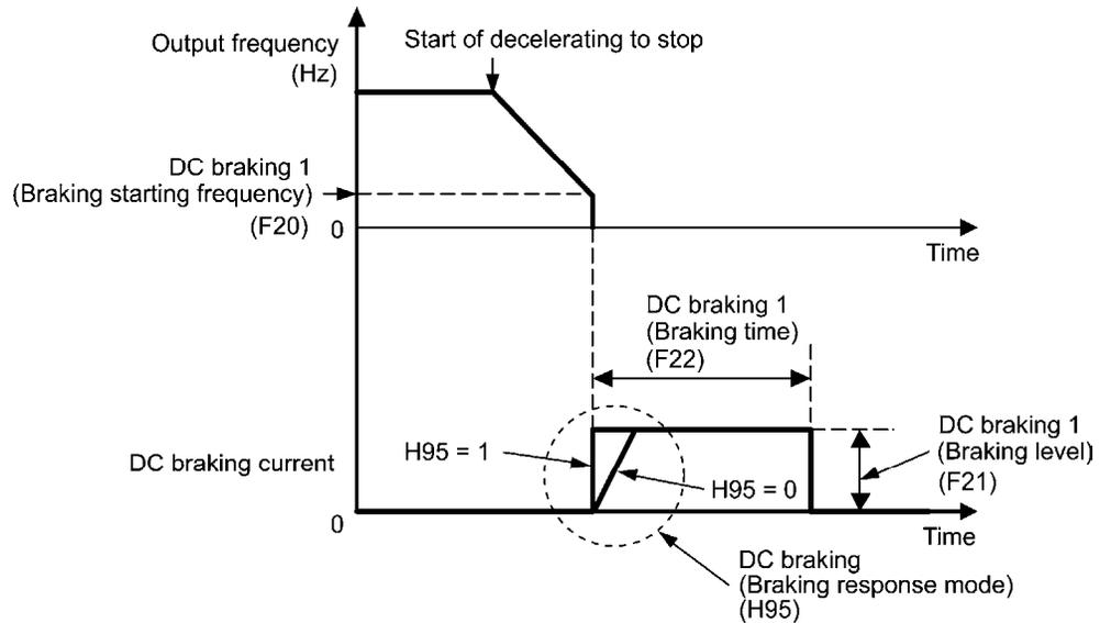
**Tip** It is also possible to use an external digital input signal as the terminal command **DCBRK** ("Enable DC braking").
