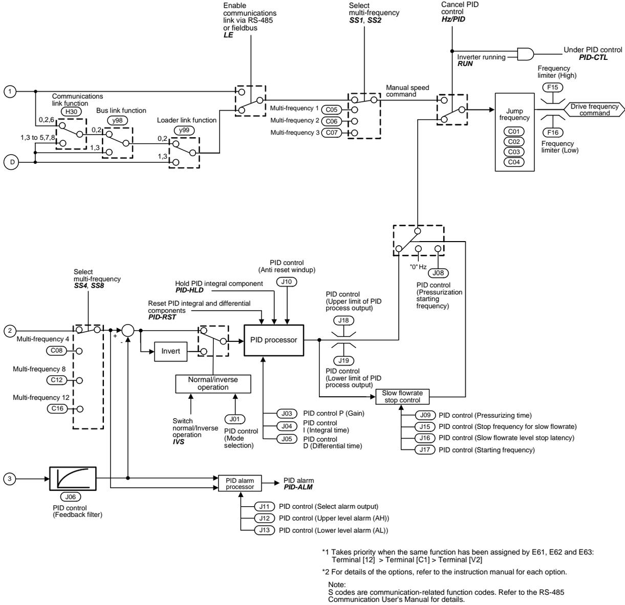
Figure 6.6 (2) PID Process Control Block
