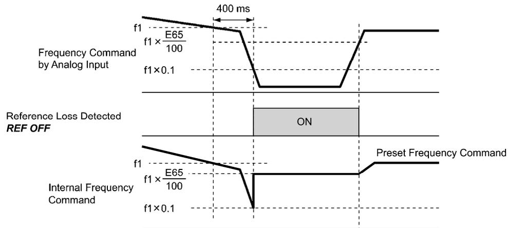
In the diagram above,  $f1$  is the level of the analog frequency command sampled at any given time. The sampling is repeated at regular intervals to continually monitor the wiring connection of the analog frequency command.
