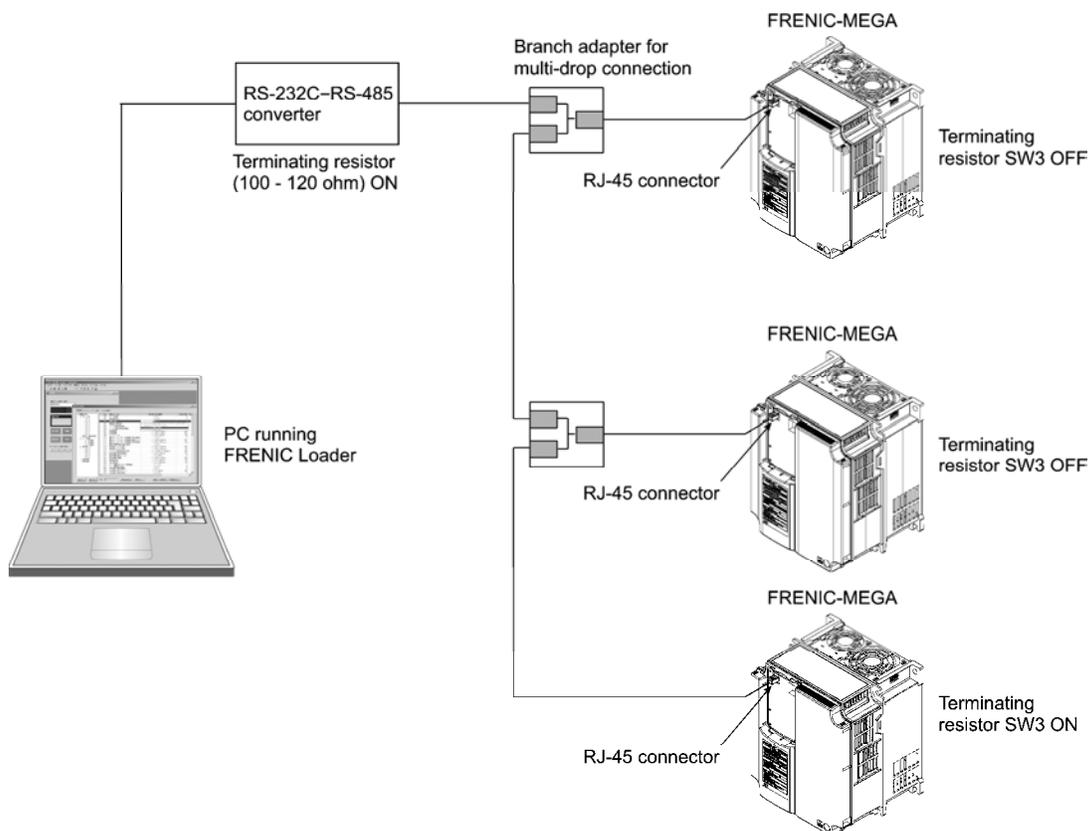
Figure 8.1 Multi-drop Connection (Using the RJ-45 connector)
