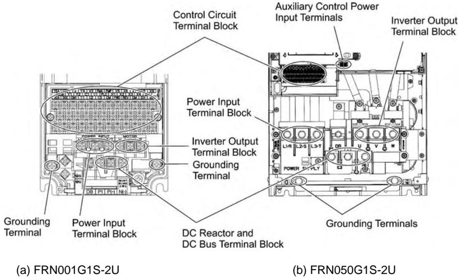
Figure 1.6 Enlarged View of the Terminal Blocks
