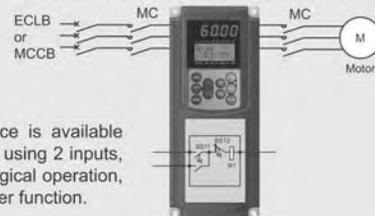
The interface is available in 10 steps using 2 inputs, 1 output, logical operation, and the timer function.
