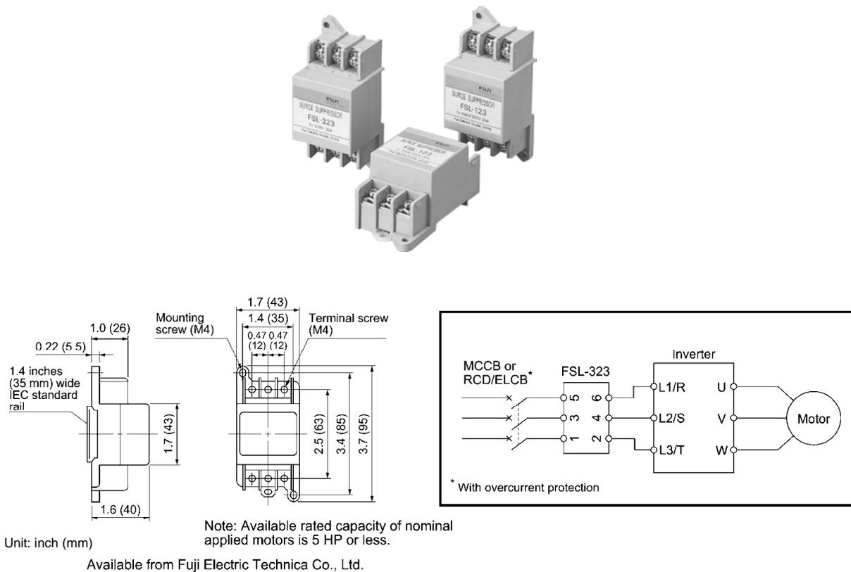
Figure 4.3 Dimensions of Surge Killer and Connection Example
