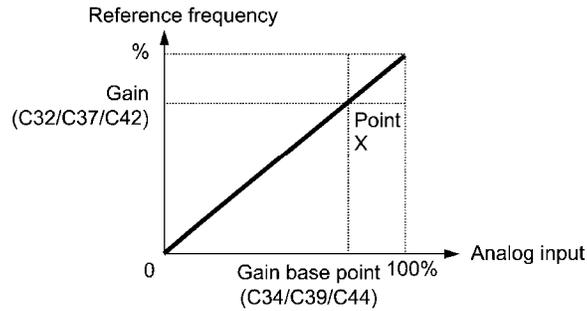
**Note** To input bipolar analog voltage (0 to ±10 VDC) to terminals [12] and [V2], set C35 and C45 data to "0." Setting C35 and C45 data to "1" enables the voltage range from 0 to +10 VDC and interprets the negative polarity input from 0 to -10 VDC as 0 V.
