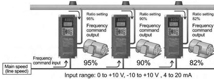
$$\text{Frequency command output} = \text{Frequency command input} \times \frac{\text{Analog input (Ratio setting)}}{100\%}$$
