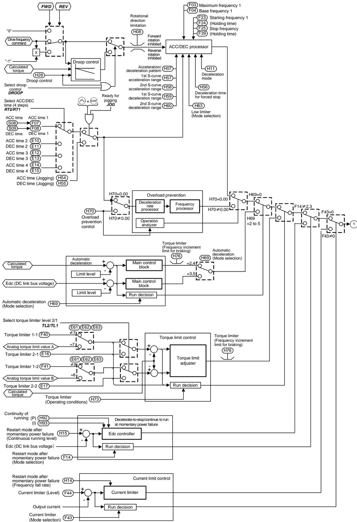
Figure 6.4 (1) Block of V/f Control with Speed Sensor
