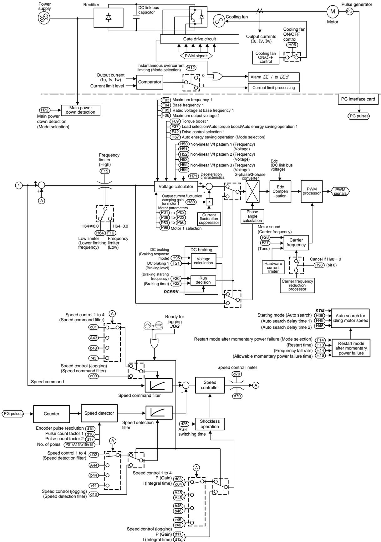
Figure 6.4 (2) Block of V/f Control with Speed Sensor
