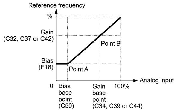
**Note** If F01 = 3 (the sum of [12] + [C1] is enabled), the bias and gain are independently applied to each of the voltage and current inputs given to terminals [12] and [C1], and the sum of the two values is applied as the reference frequency.
