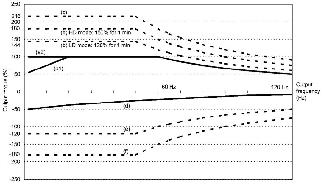
Figure 3.2 Output Torque Characteristics (Base frequency: 60 Hz)
