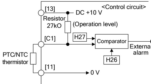
**Note** When using the terminal [C1] for PTC/NTC thermistor input, also turn SW5 on the control printed circuit board to the PTC/NTC side. For details, refer to Chapter 2, "SPECIFICATIONS."
