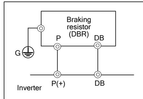
Figure 4.7 Braking Resistor (Standard Model) and Connection Example
